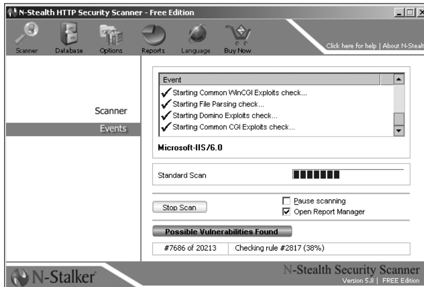
Figure 8-2: The N-Stealth port scanner has identified that this particular target computer is running Microsoft IIS, version 6.0.
