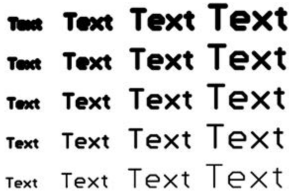
Figure 5-7: Silkscreen legibility at various text heights (40, 60, 80, and 100 mils) and line widths (8, 12, 16, 20, and 24 mils)
