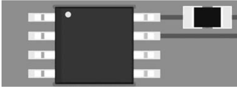
Figure 5-3: A circuit with solder mask
