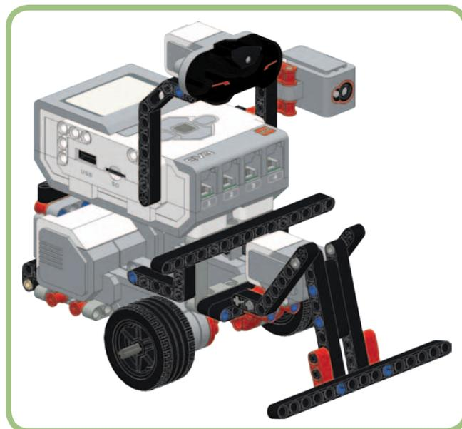
Figure 6-21: TriBot configuration for the BumperBot3 program
