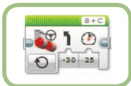
11. Select the Move Steering block on the lower Sequence Beam, and set the mode to **On**.
