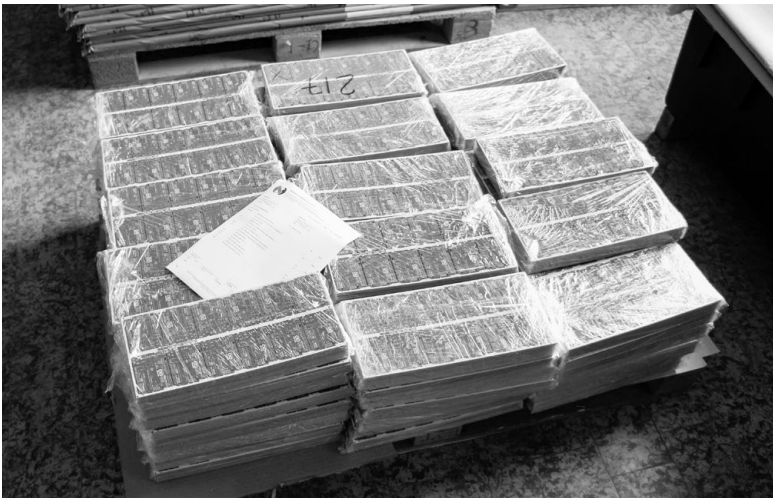
A veritable stack of about 25,000 bare Arduino PCBs, ready to leave the PCB factory. From there, they were stuffed, shipped, and sold to makers around the world!
