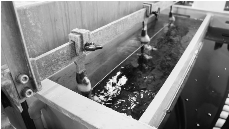
A machine that moves panels around in etchant
