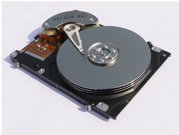
Figure 7-3: A photograph of an opened hard disk drive, showing the disk heads; photo credit: Geni, license: CC BY-SA 3.0 via Wikimedia Commons; https://upload.wikimedia.org/wikipedia/commons/d/dc/MPC310AHard_drive.JPG
