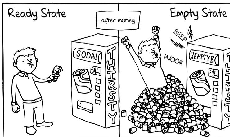
Consider the ubiquitous soda machine. Initially, it is full. You put in a dollar bill, and the machine responds by dispensing a can of soda. The machine is now in a different state; it is partially empty. Eventually, it will dispense its last can and enter its final state, the empty state. Think of Hungry Henry's state machines like this, but with less liquid and more cupcakes.
