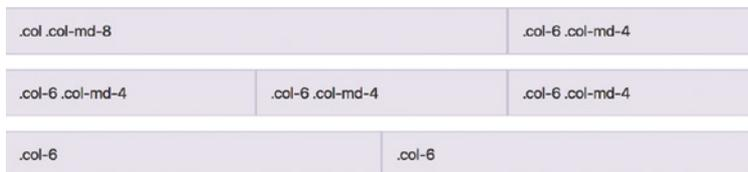
FIGURE 2-9: Some of the CSS classes included in Bootstrap to align and set your objects in the underlying grid.
