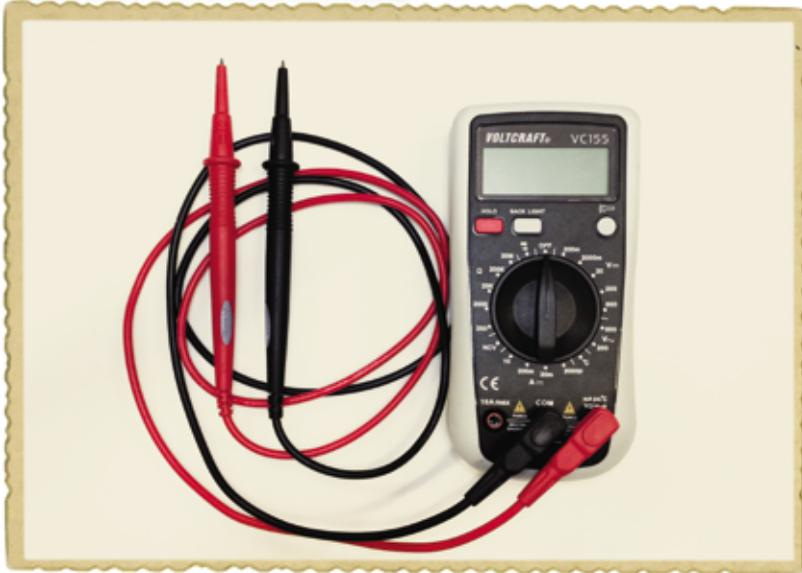
The red lead is the positive lead, the black lead is the negative lead, and the big dial in the middle lets you tell the multimeter what to measure. If you're having problems with a circuit, measuring the voltage at key points in your circuit is one practical way to figure out what's wrong.
