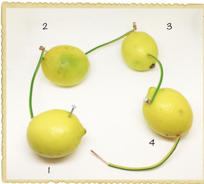
When you connect batteries in series, you can add their voltages to find your total. Four 1 V lemon batteries should give you 4 V. If you have a multimeter, measure the voltage between the two ends to see whether everything is connected. You should get a voltage of around 3.5 to 4 V.
