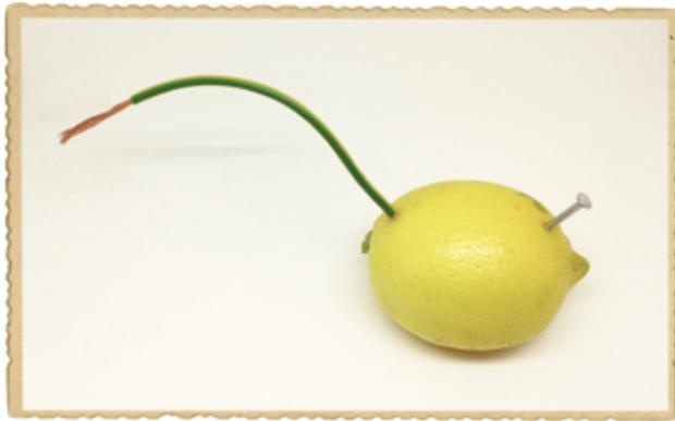
Get your multimeter, set it for DC voltage measurement, and test your lemon battery now. Place the positive test lead on the copper wire and the negative test lead on the nail. If everything works correctly, you should see a voltage of around 1 V on your multimeter.
