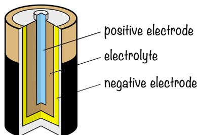
You can actually make your own battery by using a simple nail for one electrode and a copper wire for the other. Stick both into a lemon, and the lemon juice is your electrolyte.
