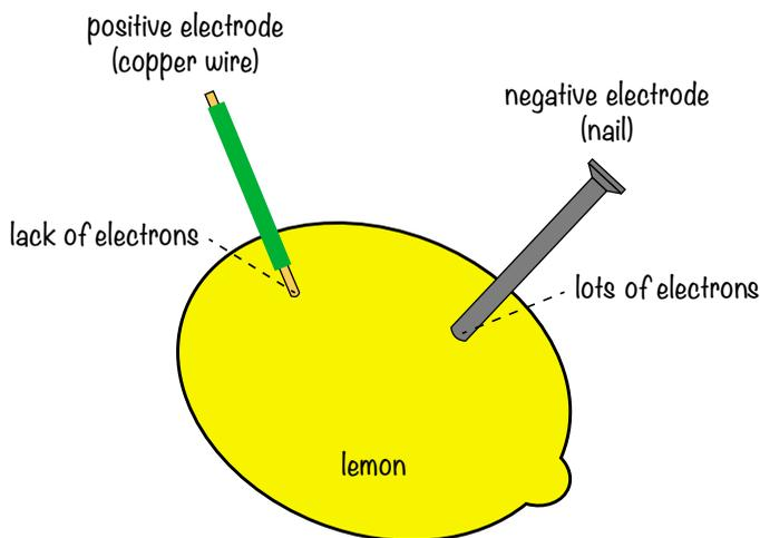
The copper wire becomes the positive terminal of the battery, and the nail becomes the negative terminal.
