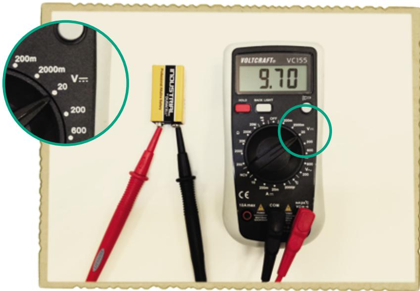
In this example, the meter is measuring the voltage between the positive and negative terminals of a 9 V battery. Notice that my dial is turned to 20 V, in the range showing a V with a straight-line symbol. But there's another V on the multimeter with a wavy line next to it. Let's look at what these symbols mean.
