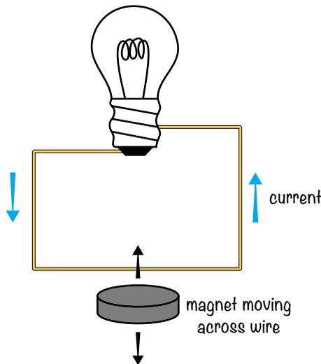
If you stop moving the magnet, the current also stops—even if the wire is still within the magnetic field—because the magnetic field is no longer changing.
