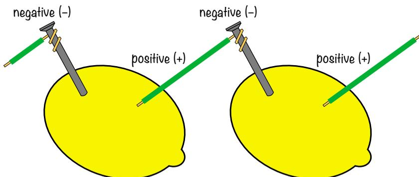
To wire four lemons in series, just repeat that process a couple more times. Line your lemons up in a row with the copper wires pointing to the right and number the lemons from 1 to 4, beginning from the left. Connect the copper wire from lemon 1 to the nail in lemon 2. Twist the wire onto the nail so that the metals connect without coming apart.
