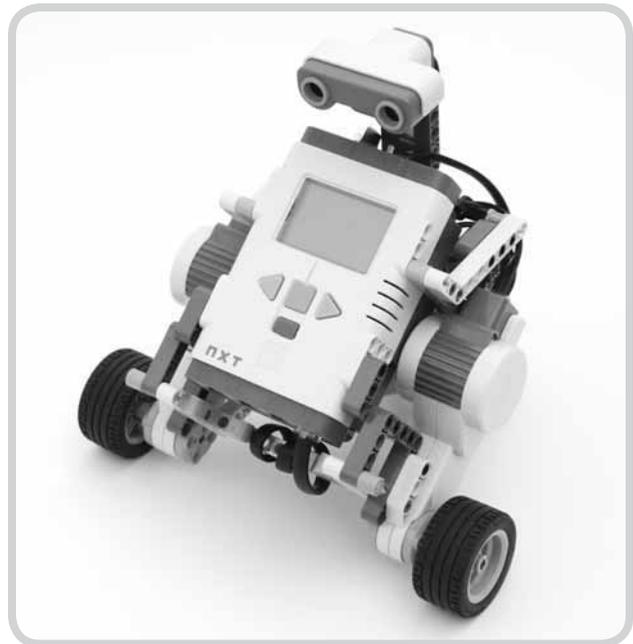
Figure 6-1: The Discovery robot: an enhanced version of the Explorer equipped with an Ultrasonic Sensor to make the robot "see"
