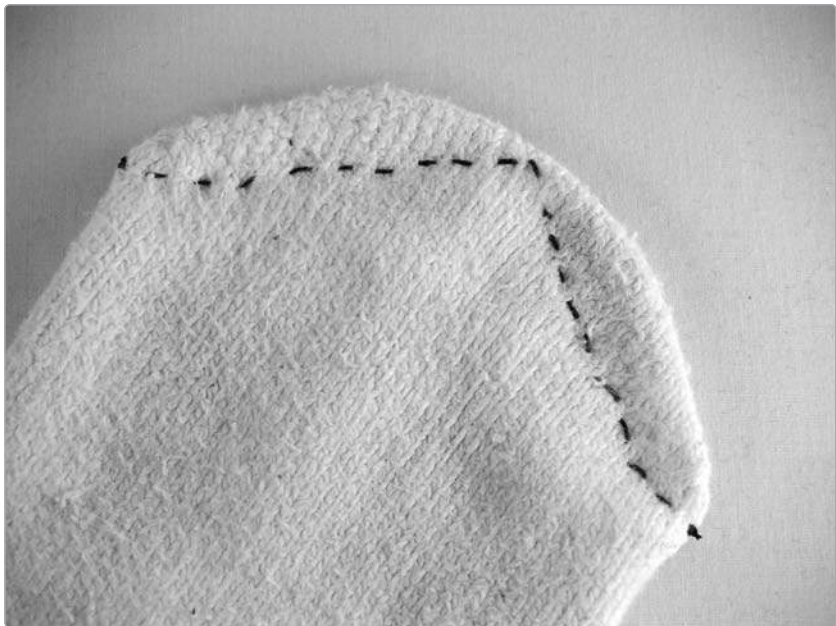
FIGURE 3-9: The mantle with fins, shown here sewn with contrasting thread for clarity
