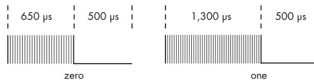
Figure 12-3: Modulated pulses in the Sony TV protocol
