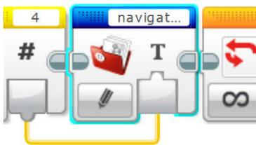
Place the File Access block after the dGPS block inside the loop and make a wire connection between the two. This will pass data from the dGPS sensor to the file. On the File Access block, set **File Access** to **Write** and **File Name** to *navigation log*.
