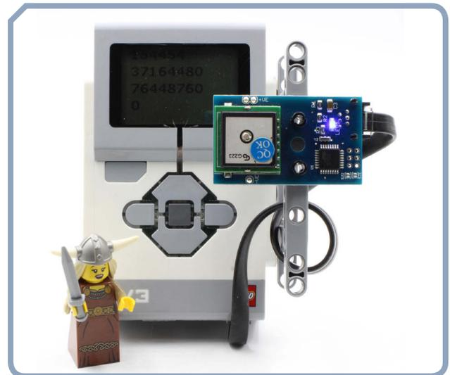
**FIGURE 3:** Attach the dGPS to the EV3 Intelligent Brick with an open center frame liftarm.
