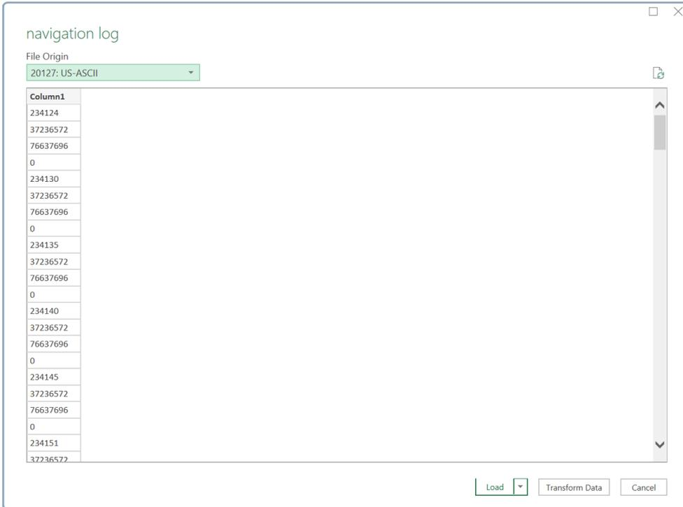
**FIGURE 6:** As the navigation log is imported into Excel, the repeated sequence of time, latitude, longitude, and velocity displays in a preview.
