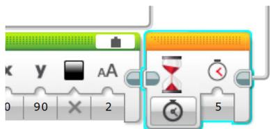
Place the Wait block after the last Display block. Set **Wait** to **Time** and **Seconds** to **5**.
