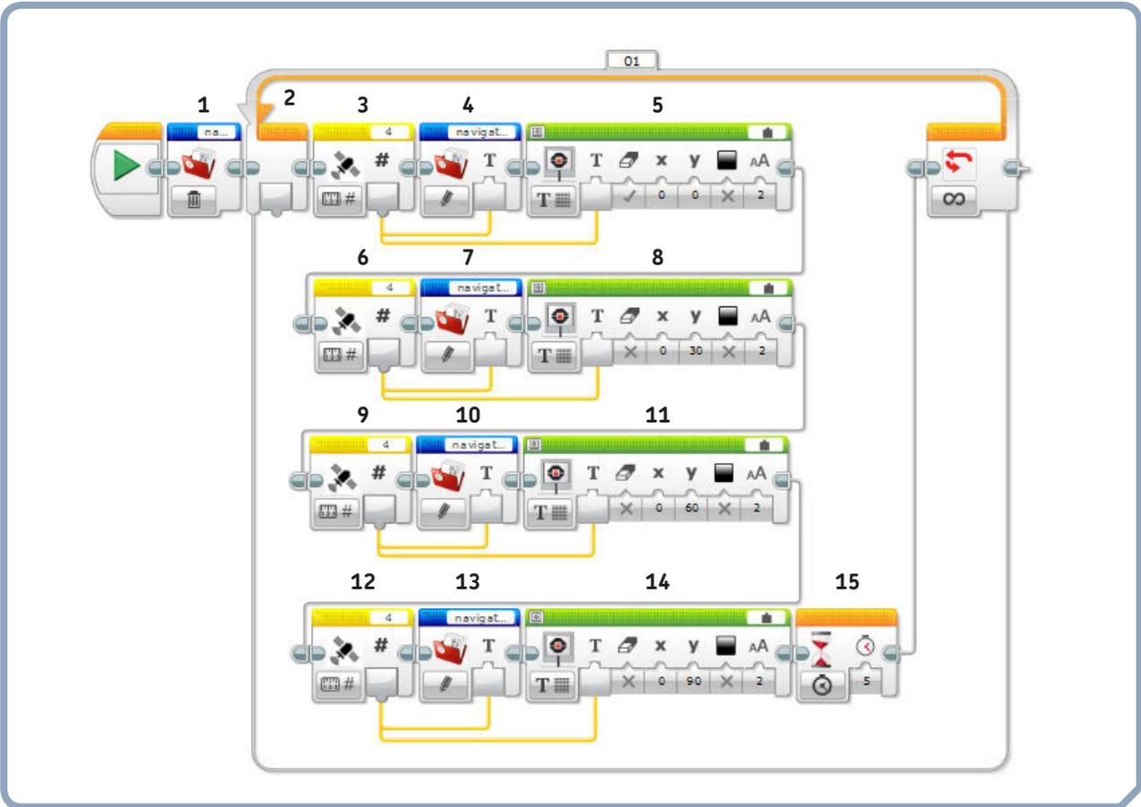
FIGURE 4: The software for the LEGO Car Tracker samples data inside a continuous loop.
