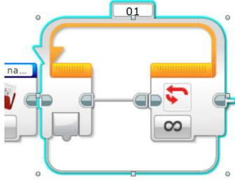
Attach the Loop block after the File Access block.
