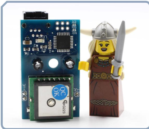
**FIGURE 1:** The antenna on the dGPS is the square component at the bottom of the circuit board.
