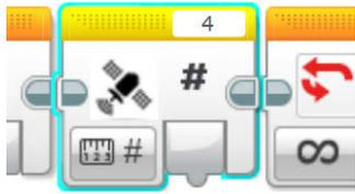
Select the dGPS block from the Sensor tab at the bottom of the screen and place it within the loop. Set **dGPS** to **Read UTC Time** and set **Port** to **4**.
