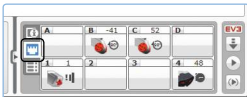
Figure 6-5: You can also view sensor measurements from within the EV3 software. If the values aren't being updated continuously, download a program to the robot to refresh the connection. Click one of the sensors to choose which type of measurement you want to see.
