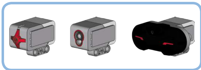
Figure 6-2: The EV3 set comes with a Touch Sensor (left), a Color Sensor (middle), and an Infrared Sensor (right).
