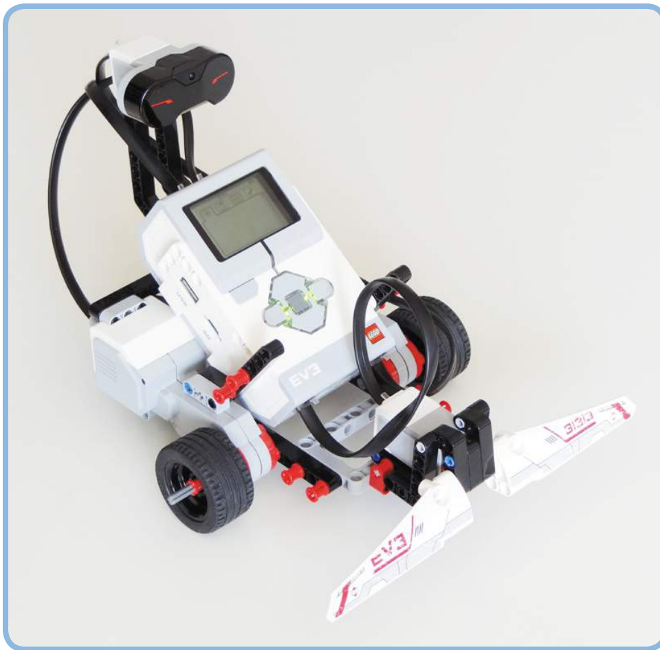
Figure 6-1: The EXPLOR3R uses a bumper with a Touch Sensor to detect objects it runs into.
