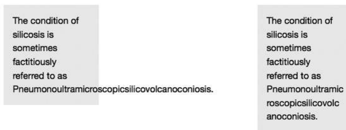
Figure 6-11: Example of text without (left) and with (right) a break-word value for word-wrap
