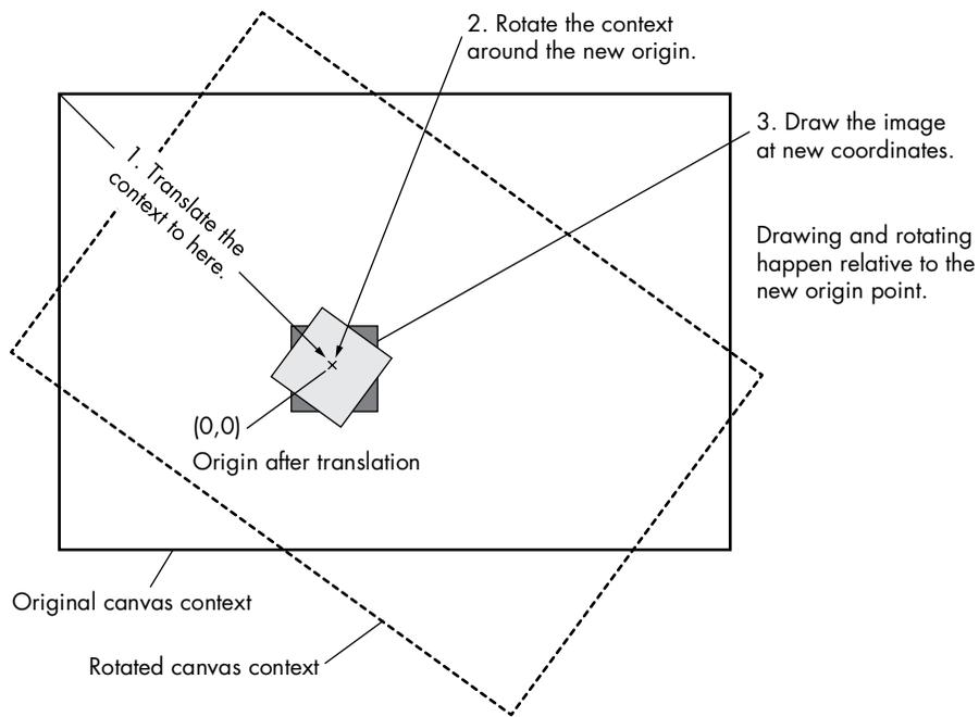
Figure 6-1: Drawing a rotated image onto the canvas
