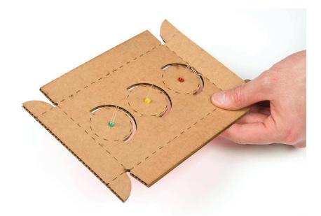
Next, bend the cardboard along the scored lines, as shown in Figure 2-19. Bend the vertical sides **1** toward the interior, and then do the same with the top and bottom sides **2** and the tabs **3**. (The sides and tabs are labeled in Figure 2-15.)
