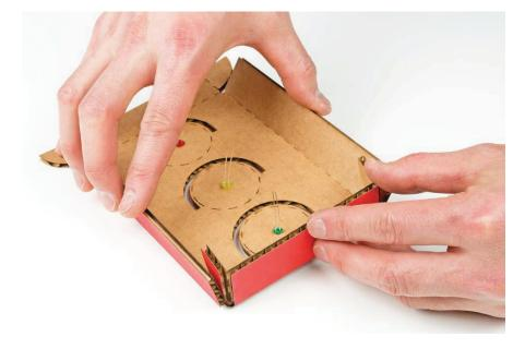
Position the tabs **③** inside the vertical sides **①**, and glue them in place as shown in Figure 2-20. You can use hot glue, tape, or craft glue—we prefer hot glue because it's easy to work with, sets quickly, and has a pretty strong bond.
