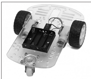
Figure 8-12: Two-wheel-drive robot vehicle chassis (PMD Way part number 72341119)
