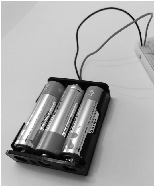
Figure B-6: Using three AA batteries to power a circuit on a breadboard
