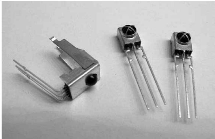
Figure 12-5: Infrared detector/demodulators
