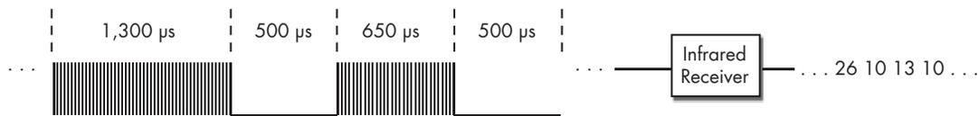
Figure 12-8: Measuring waveform timing in external hardware
